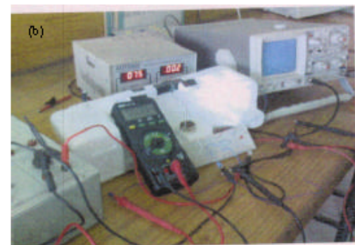
Fig. 7: Switching behaviour of soil transistor/NOT logic
