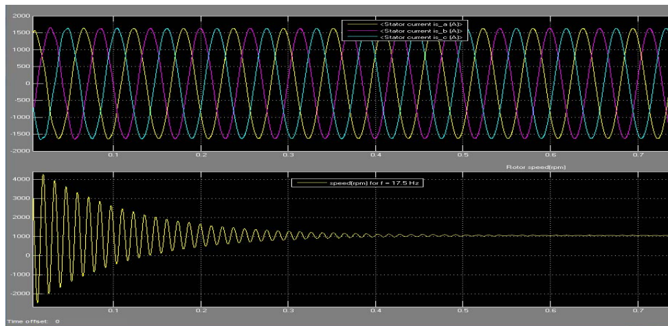
Fig. 24: Phase Currents and speed at f = 49.3 Hz
