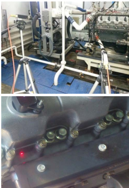
Fig. 14: Installation of laser vibrometers (left) and place the guidance of the laser vibrometer at the head of the gas engine block (right)
