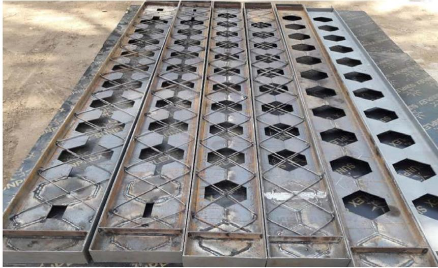
Fig. 2: Fabricated castellated steel beams
