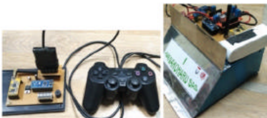
Fig. 9: Implementation Sumo robot system
