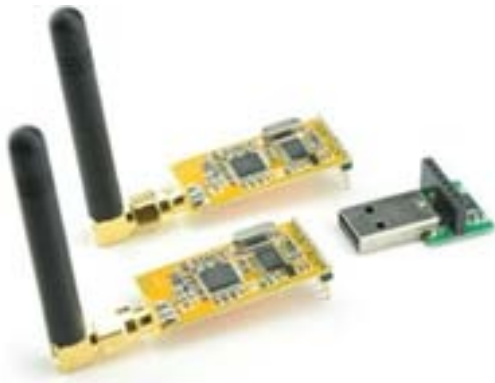
Fig. 5: APC220 module communication (Yamato et al. , 2008)
