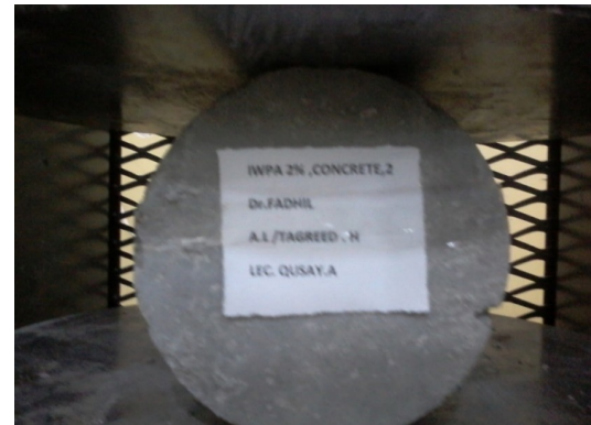
Fig. 3: Cylindrical IWPA concrete specimen under tensile test
