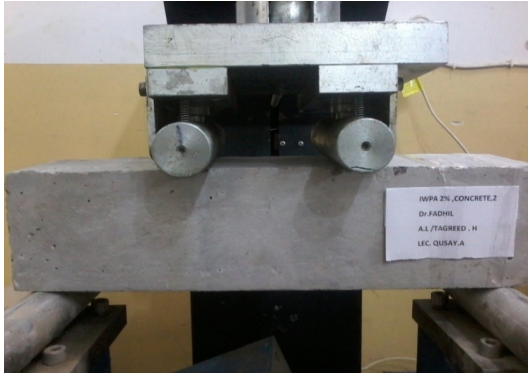
Fig. 4: Beam concrete specimen under third point flexural test
