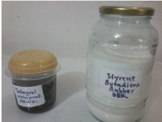
Fig. 1: Integral water proofing admixture and SBR latex used in the study
